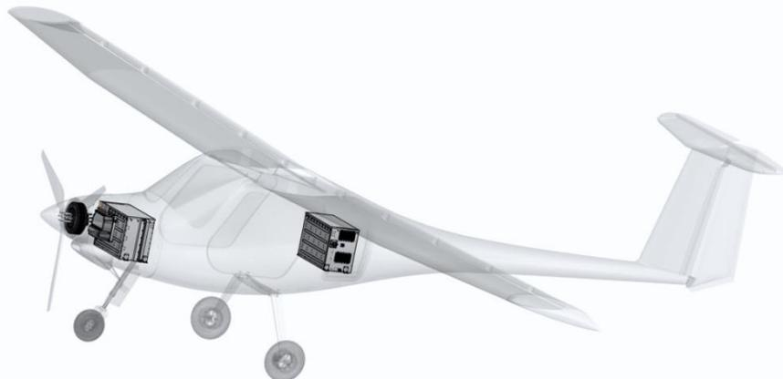
The holy grail for zero emission airplanes is the direct electric powertrain. Many developments are underway and the first airplane - the Velis-Electro from Slovenian company Pipistrel - is EASA certified. Designs not conceivable before will come with multiple computer controlled engines and induce novel airplane.
