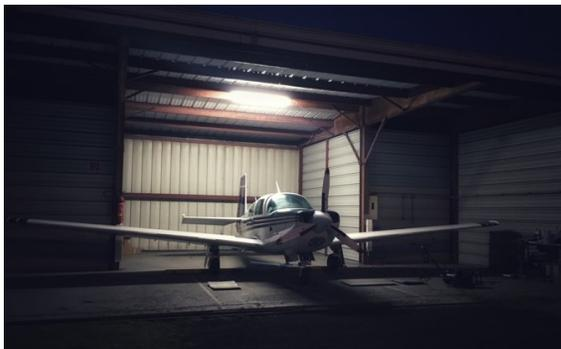
This Mooney is powered by a flat six-cylinder Continental 210 hp TSIO-360-LB turbocharged engine, driving a 3-blade McCauley propeller. The M20K was introduced as the fastest single-engine production airplane in the world. From 1979 to 1985, a total of 888 units of M20K 231 have been produced.
